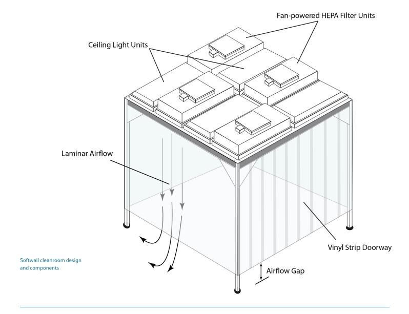
is too small, the air will push the panels outward to an unacceptable distance and inhibit good laminar airflow. If the gap is too large, the cleanroom will not keep enough positive pressure to push contaminants out.
